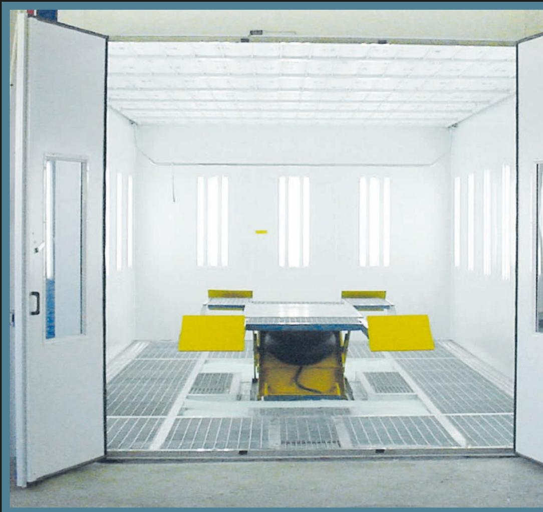
*The Stratos spray booth was born from the needs of our customers. Its vertical lighting guarantees an extended filtering plenum surface.*
